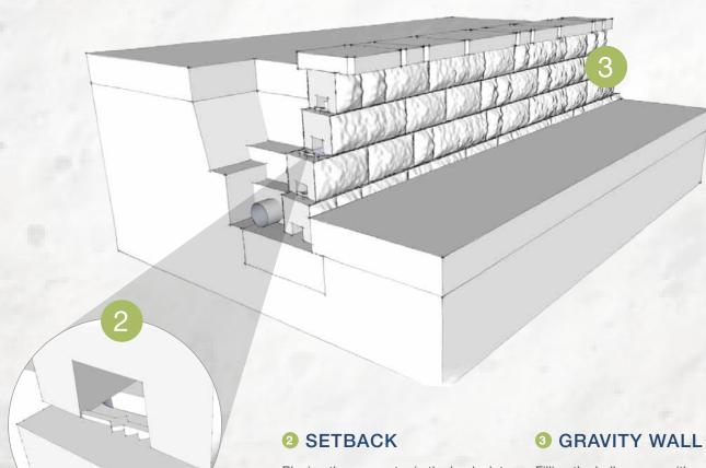
Placing the connector in the back slot will give every row batter/setback. The middle slot will be vertical or no batter/setback.
