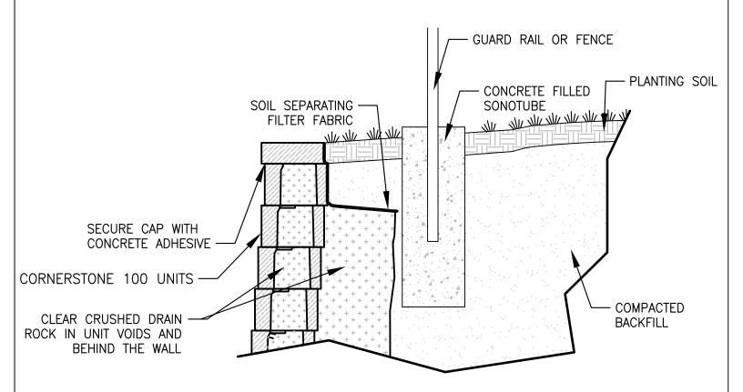
NOTE: SONOTUBES ARE PLACED DURING CONSTRUCTION. DISTANCE FROM FACE OF WALL & DEPTH OF SONOTUBE VARY WIND LOADS AND LATERAL LOADS HAVE NOT BEEN CONSIDERED. COSULT A QUALIFIED ENGINEER
