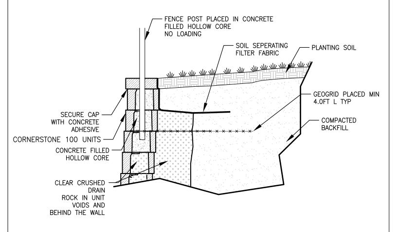
NOTE: CONCRETE CORE FILL MIN 3 UNITS DEEP ALONG THE FULL LENGTH OF WALL WITH A 4.0FT MIN LENGTH GEOGRID AT THE SECOND LAYER.
